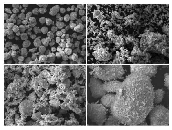
Fig. 5 Microscopy images for four UF<sub>4</sub> samples of differing origins. Adapted from Ref. [49]
