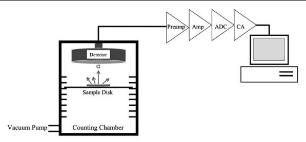
Fig. 3 Representation of an alpha spectrometry system, including associated electronics and recording devices
